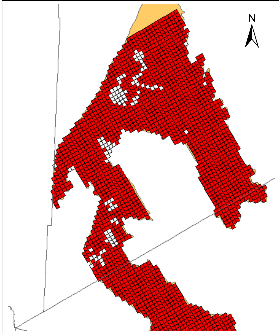
Figure 1. Extent of the Salt Basin Bolson aquifer in the GAM. Model cells in red are active cells that contain pumpage in 2000. Model cells in white are active cells without pumpage. The actual extent of the Salt Basin Bolson aquifer is shown in tan.
