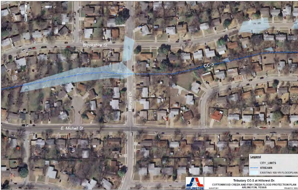
Figure 11: 100-YR Flood Plain Tributary CC-3 at Hillcrest Drive
