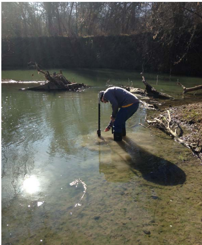
Figure 10. Crew member installs a stream level logger.
