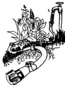
Drip irrigation soaks the root system without any runoff
