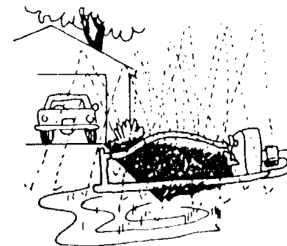
Incorrect location for the sprinkler = wasted water
