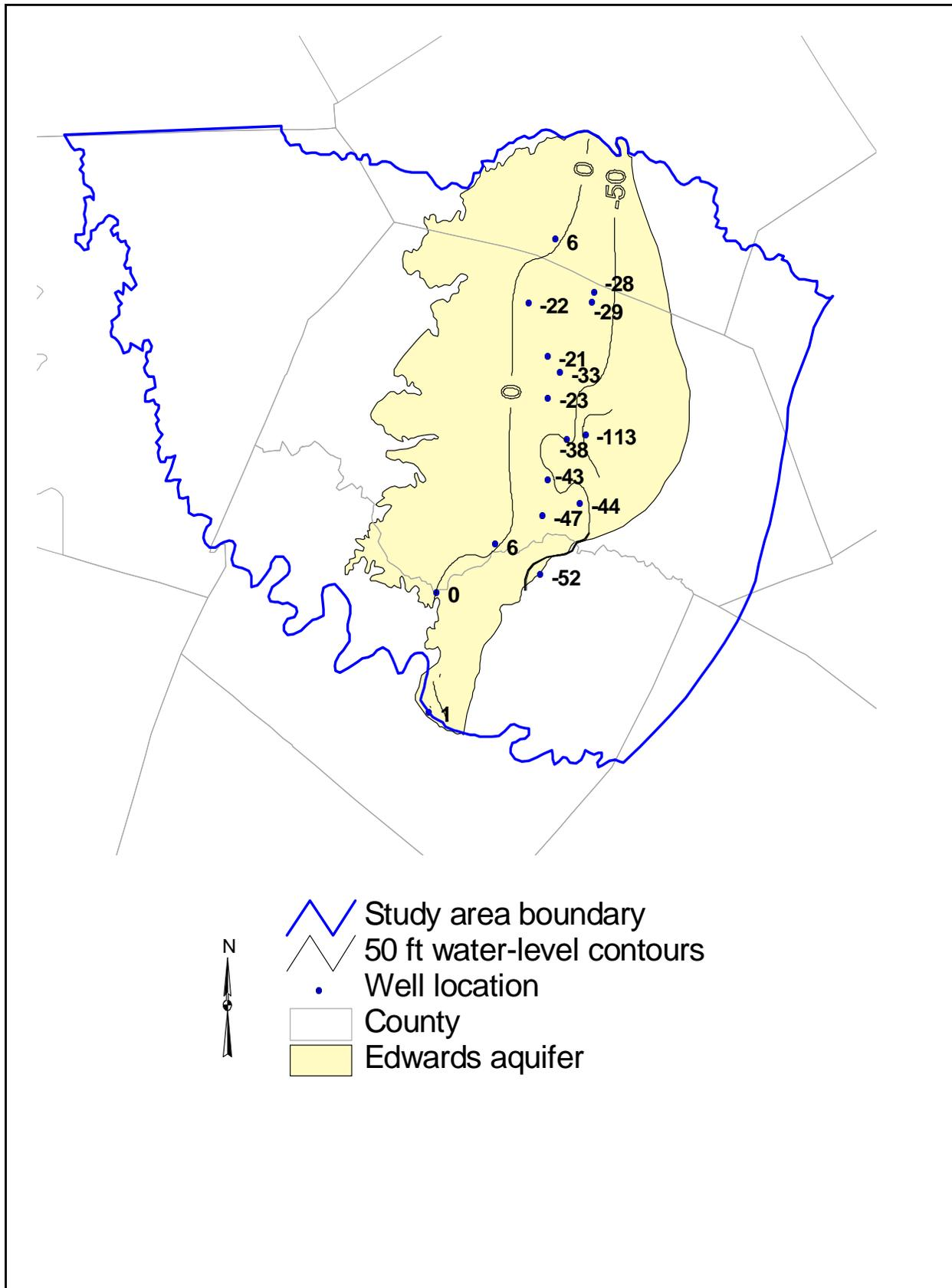
Figure 5. Water-level changes in the Edwards aquifer based on data collected 1987-1988 and data collected 1997-1998.
