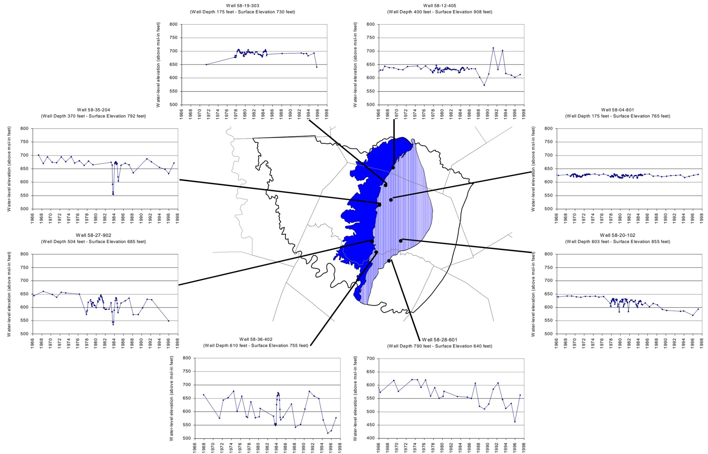
Figure 3. Water-level hydrographs for selected wells completed in the Edwards aquifer.
