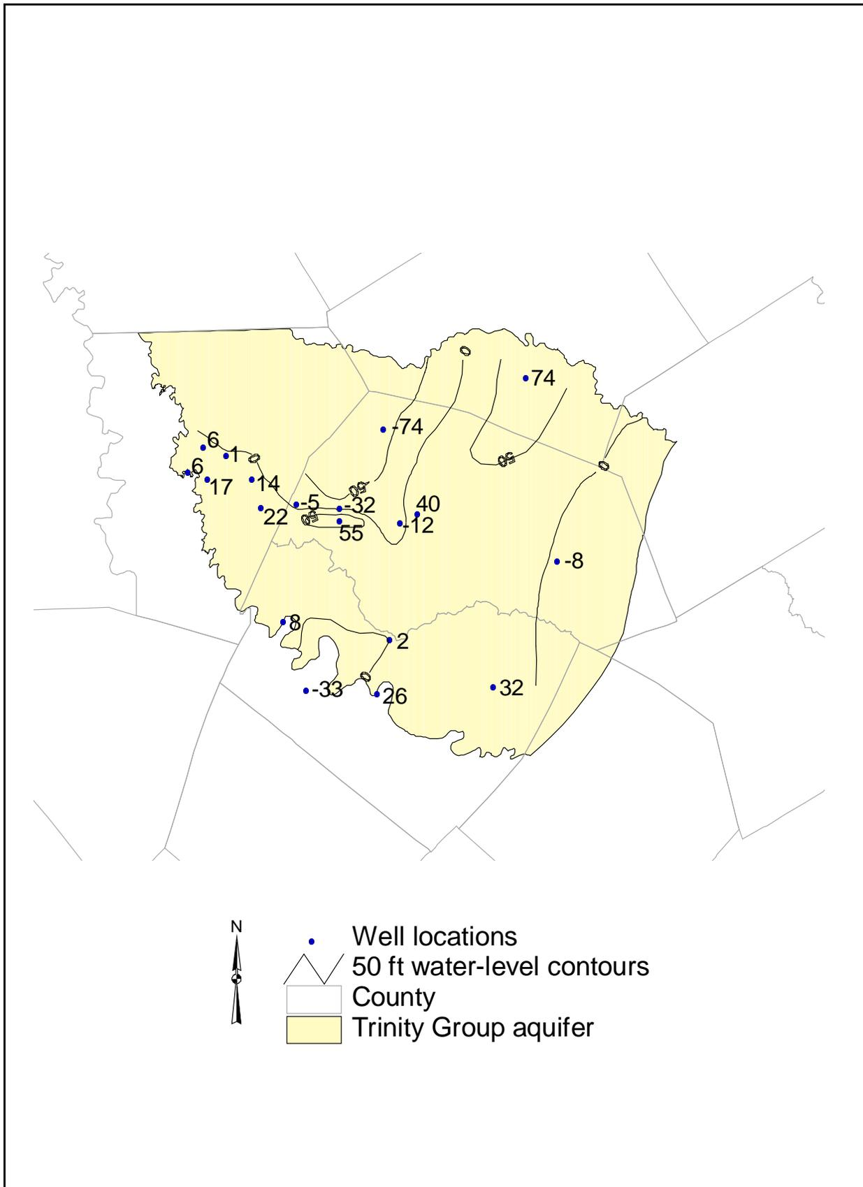
Figure 8. Water-level changes in the Trinity Group aquifer based on data collected 1987-1988 and data collected 1997-1998.
