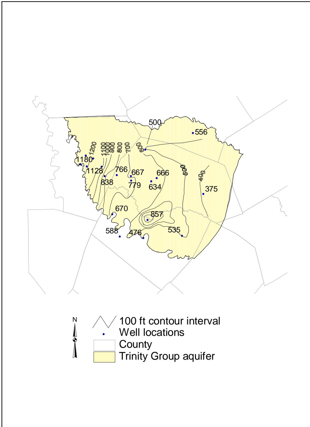
Figure 7. Potentiometric surface map for the Trinity Group aquifer from data collected 1997-1998.
