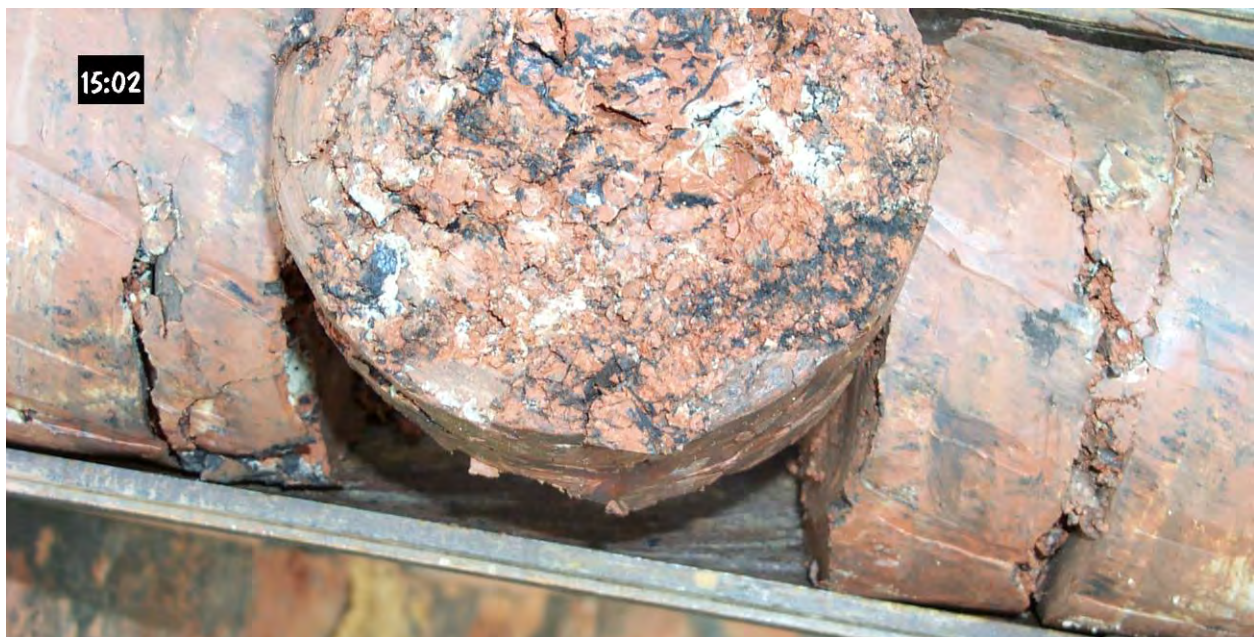
Figure 2-15. Photograph of a core of the Beaumont Clay at a depth of about 30 feet from a well near Houston. Whitish areas are carbonates, darker areas are organic matter, and pinkish (gray) areas are clay. Note tightness of the clay that retards any significant infiltration of recharge.
