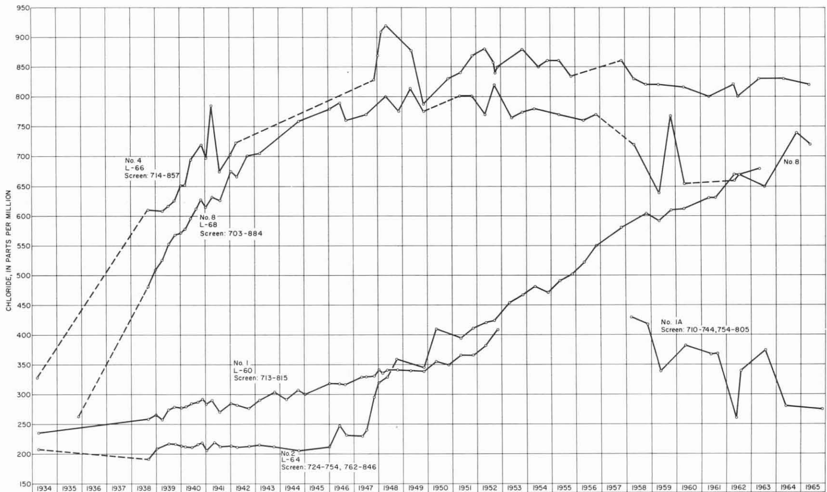
Figure 16 Changes in Chloride Content of Water from Wells in the City of Galveston's "Old" Well Field in the Vicinity of Alta Loma
