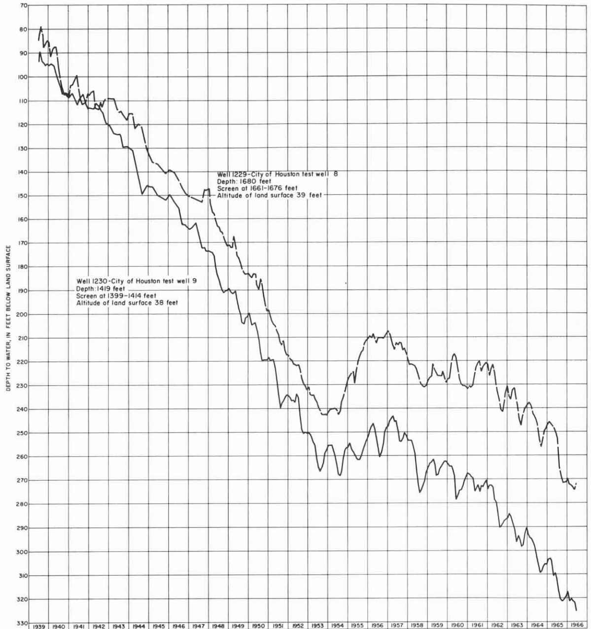
Figure 9 Changes in Water Levels in Two Single-Screened Deep Wells in the Southern Part of the Pasadena Area
